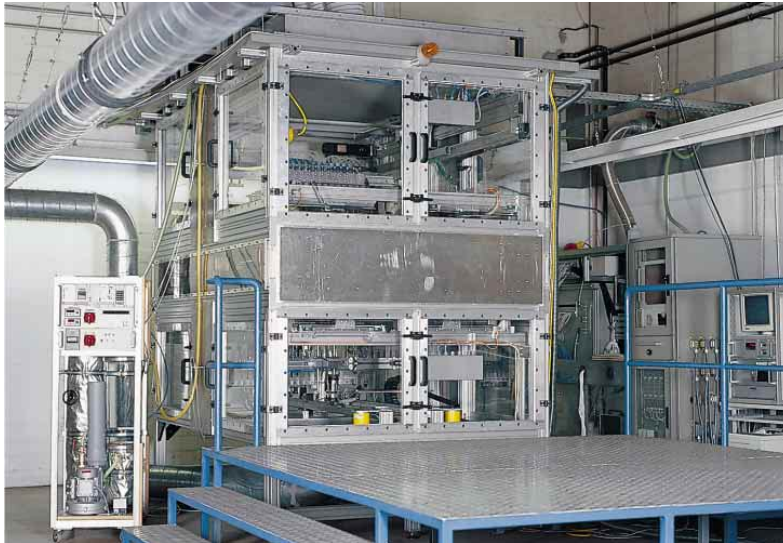
Multi-scanner for HEPA and ULPA filters
